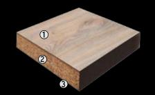
1. PVC Top layer 2. High density chipboard. Thickness 38 mm 3. Aluminum foil
