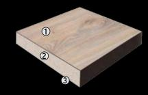
1. PVC Top layer 2. Calcium Sulphate. Thickness 30 mm 3. Aluminum foil
